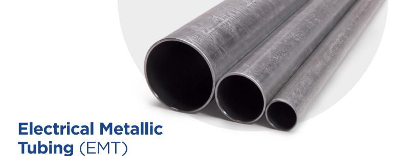
To manufacture our high-quality EMT, we use low-carbon strip steel that is electric-resistance welded into tubing and then in-line galvanized for superior rust protection. The conduit is then coated with a low-friction organic polymer inside and out to resist corrosion and make feeding wires easier. Before leaving our facility, our EMT undergoes testing to ensure it bends without kinking, flattening, flaking or cracking.
