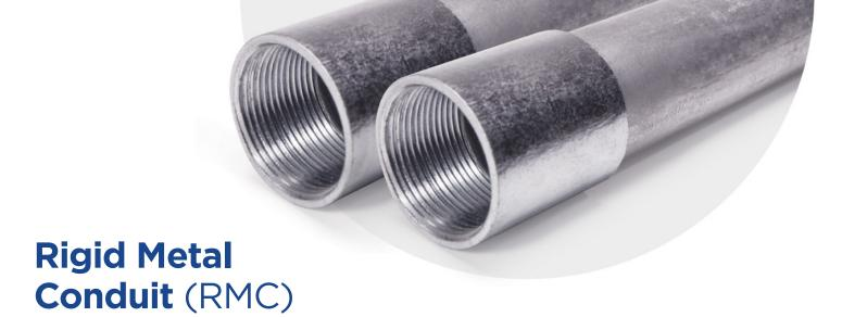
Manufactured as the heaviest-gauge tubing available, RMC stands up to the most challenging physical environments. Our RMC is hot-dip galvanized and then coated in layers of chromate conversion and organic polymer for extra protection. This makes it especially strong and resistant to environmental and mechanical corrosion. A number of rigorous quality verifications must be passed—including bend and thread testing—before any RMC is approved to leave our facility.
