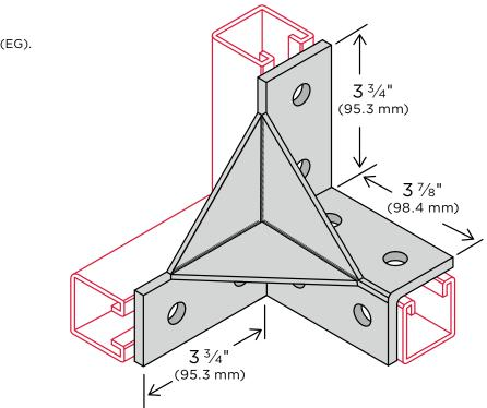
Material is 1%" (41.3 mm) wide x ¼" (6.3 mm) thick unless specified. Holes are %\*" (14.3 mm) diameter, 1%\*" (20.6 mm) center to edge on 1%\*" (47.6 mm) centers unless specified.
